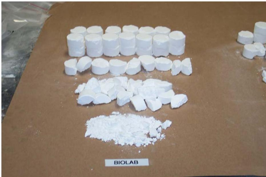
40 tablets were dropped from 4 ft onto an iron table. Resulting classes were: (1) powder, (2) small pieces and broken tablets (this class is further split in the picture into small pieces and large pieces, and (3) whole unbroken tablets
